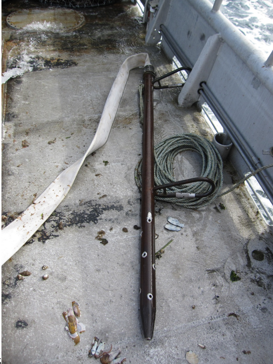
Figure 1. Pot pump used to recover buried or sanded-in pots.
